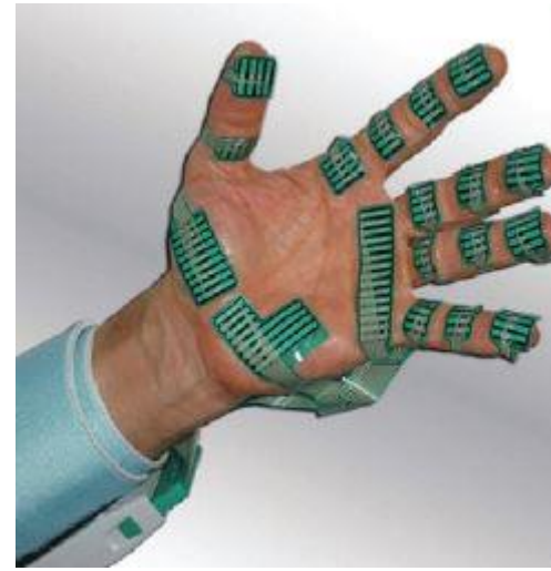
Figure 2. Pressure sensors used to line work gloves
